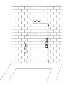
2) Installation of charging pile inlet
